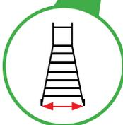
**Base width** is also very important because as ladders get taller, the base width increases. It is important to be sure that the ladder will not be too wide for your workspace. We offer different tread widths to accommodate most work areas.
