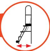
**Base length** is the measurement of how long the base of the ladder runs. This is dependent upon the height of the ladder. The taller the ladder, the longer the base.
