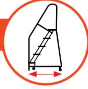
**Base length** is the measurement of how long the base of the ladder runs. This is dependent upon the height of the ladder. The taller the ladder, the longer the base. Also lower climb angles increase base length.
