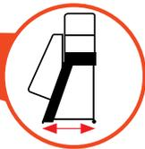
**Base length** is the measurement of how long the base of the ladder runs. This is dependent upon the height of the ladder. The taller the ladder, the longer the base.
