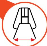
**Overall length** is the measurement between the floor-mounting brackets. This is dependent upon the height of the bridge. The taller the bridge, the longer the overall length. Lower climb angles also increase overall length.
